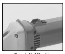
Figure 2. ON/OFF switch.
